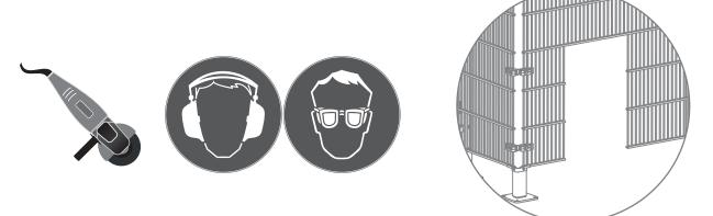
The size and position of the openings must not compromise the stability of the mesh elements.
