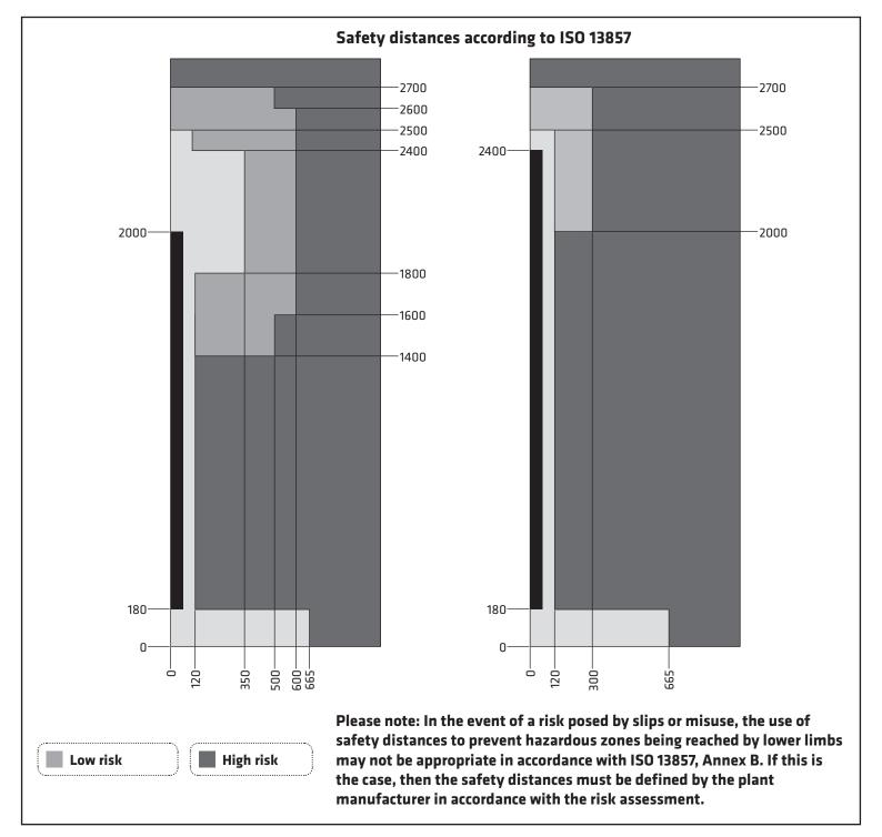
Safety distances only apply with the use of ECONFENCE® mesh elements with a mesh size of 19/190 mm. Information on dimensions and weight specifications of the system components can be found in Section 1. Technical data, page 4–5.
