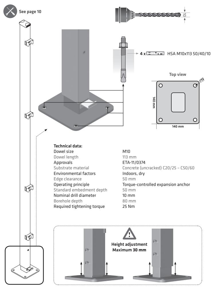
Installation of clamping element ZB31004
